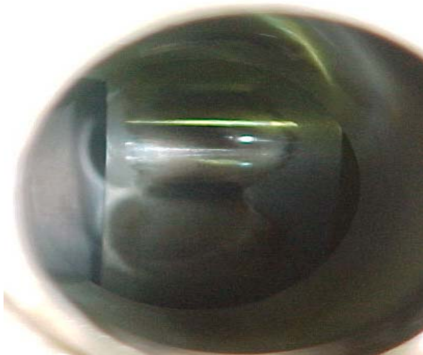
FIGURE 10 CAM LOBE APEX IN INSPECTION LOCATION (Normal wear signature shown)
