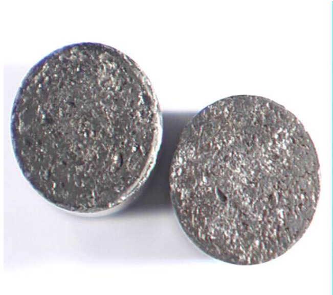
FULL FACE SPALLING
