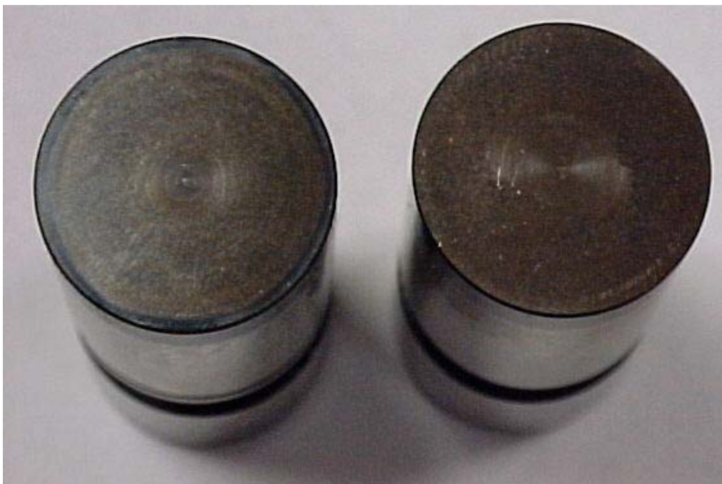
FIGURE 5 TYPICAL LIFTER FACES FROM SERVICE
