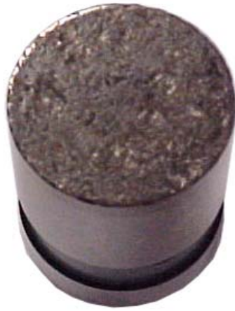
FIGURE 9 REPLACEMENT SIGNATURES, SPALLED LIFTER
