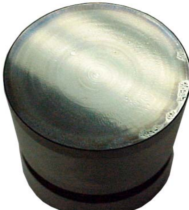
FIGURE 8 ACCEPTABLE LIFTER FACE SIGNATURE
