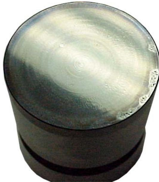
**FIGURE 6 MINOR SPALLING**
