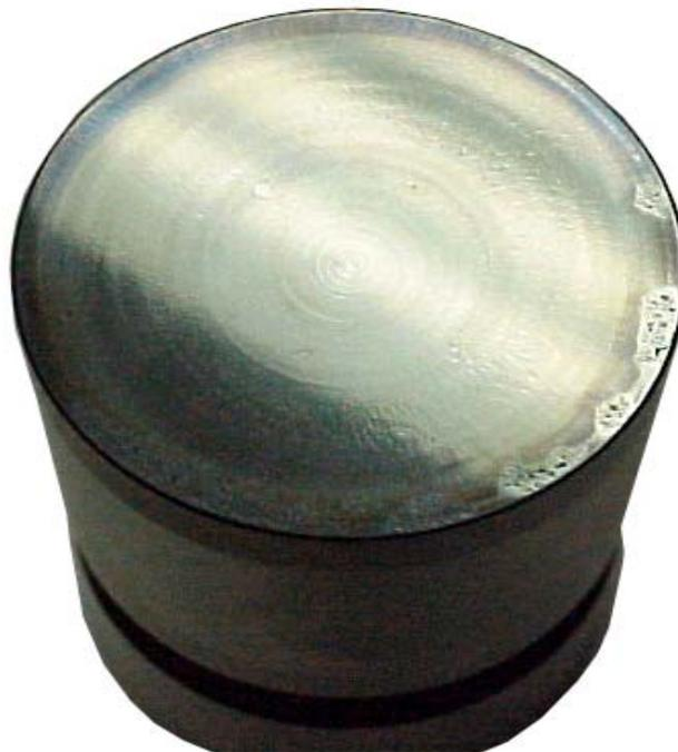
**FIGURE 8 ACCEPTABLE LIFTER FACE SIGNATURE**
