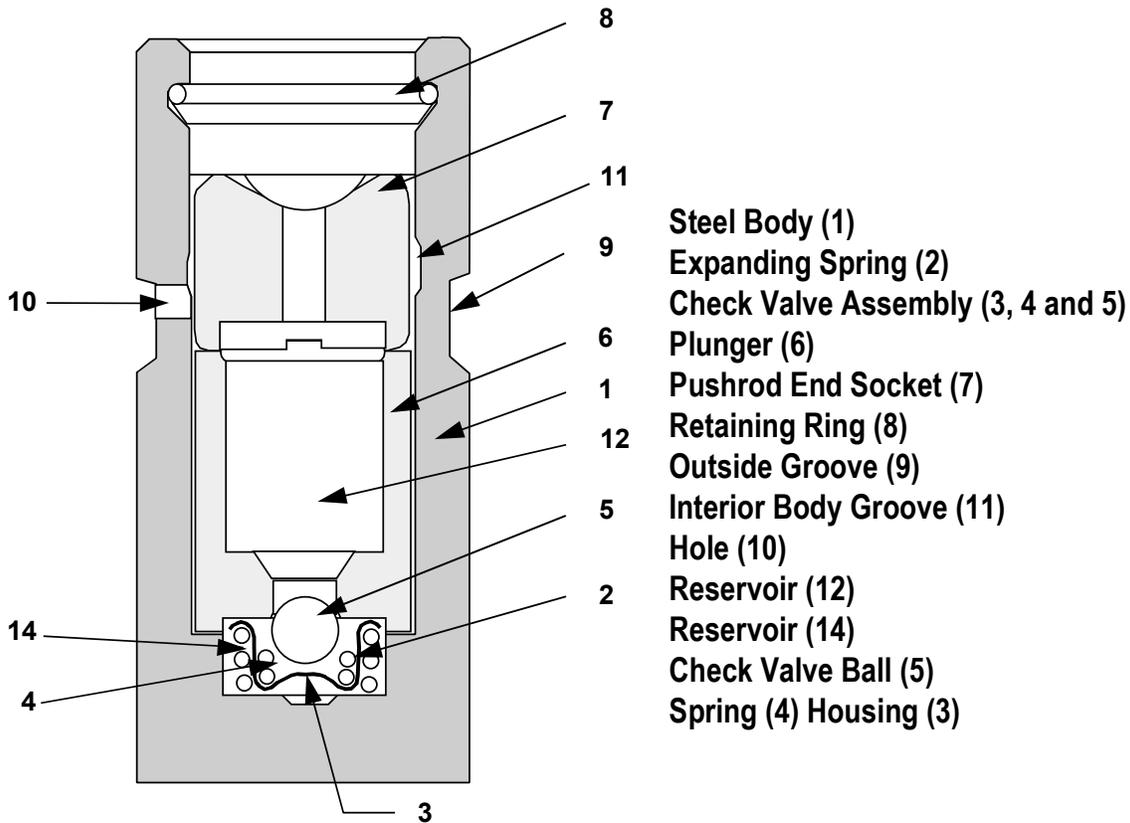
**FIGURE 2 HYDRAULIC LIFTER CROSS SECTION**
