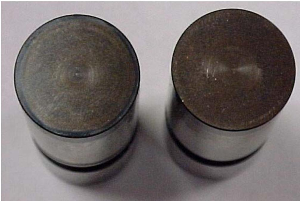
**FIGURE 5 TYPICAL LIFTER FACES FROM SERVICE**
