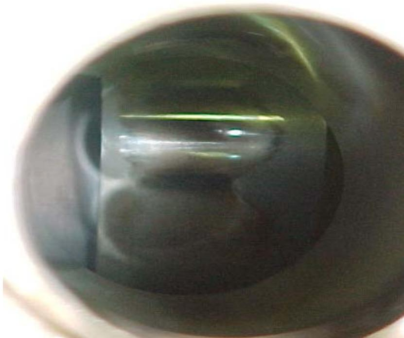
**FIGURE 10 CAM LOBE APEX IN INSPECTION LOCATION**
